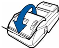
8. Tear the paper off against the serrated metal strip in the printer.
